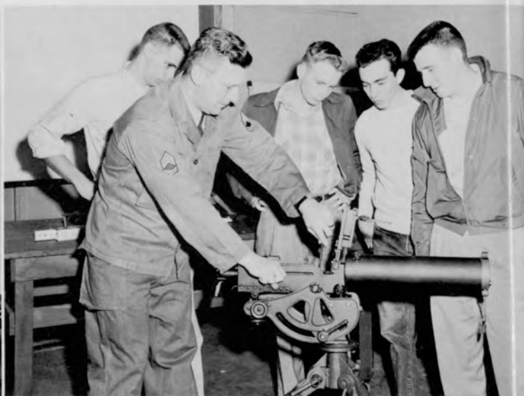
Sgt. Oplinger demonstrates bolt action of .30 calibre water-cooled heavy machine gun.
